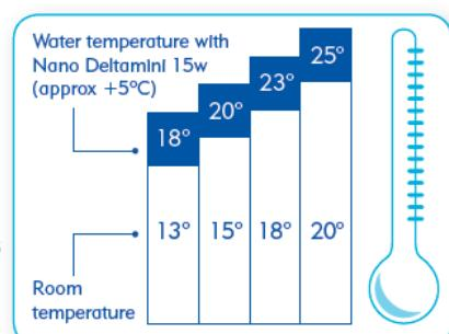
**Top Tip:** if the room ambient temperature rises above 24 degrees, turn off power to the Deltamini until the room ambient temperature returns to a temperature of 24 degrees Celsius or less.
