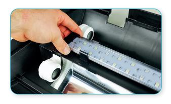
Place the Eco-Max LED in the desired location under the hood and draw around the brackets with a pencil to indicate their position.
