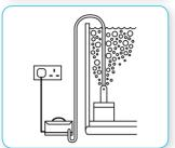
Note: if being used with a marine aquarium, we would recommend to always place the air pump higher than the water level, and use an Interpet Check Valve.
