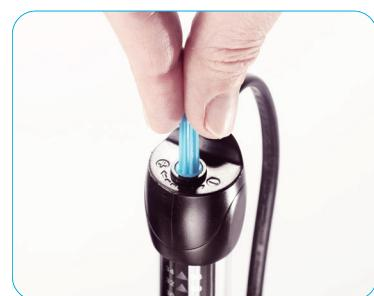
Using the suckers provided, install the heater into the aquarium in an area of high flow and ensuring it is positioned below the minimum water line of the aquarium. Position the heater at a 45° angle to get the best heating affect.
