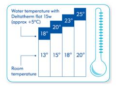
Top Tip: if the room ambient temperature rises above 24 degrees, turn off power to the Deltatherm flat heater until the room ambient temperature returns to a temperature of 24 degrees Celsius or less.
